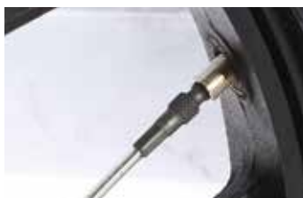
Installs valve neck on rim in correct position
