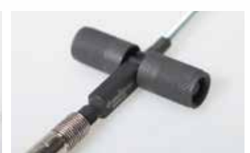
Valve thread chaser removes foreign material
