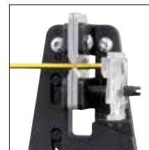
Cable is accurately positioned at length stop
