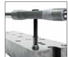
Setting the extractor with a tap wrench
