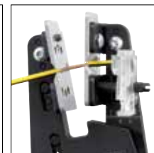
Stripping is made easy with the precision made profile blades
