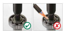
Heating up bearing will cause heat to transfer and damage tool  $% \left\{ \left( 1\right) \right\} =\left\{ \left($
