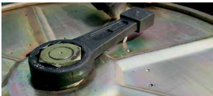
Ideal for loosening large nuts when extra force is required
