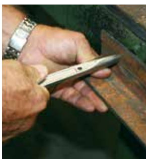
Bolt hole alignment
