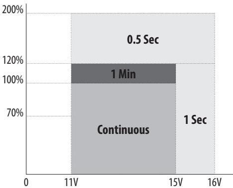
Figure 1 : Output power vs,input voltage
