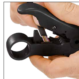
Stripping of flat cables
