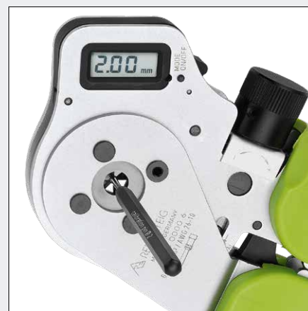
Pliers can be calibrated by the user
