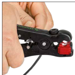
Trimming coax cables
