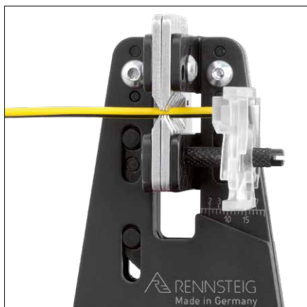
Position cable at length stop
