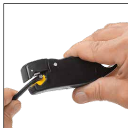
Inserting a coax cable
