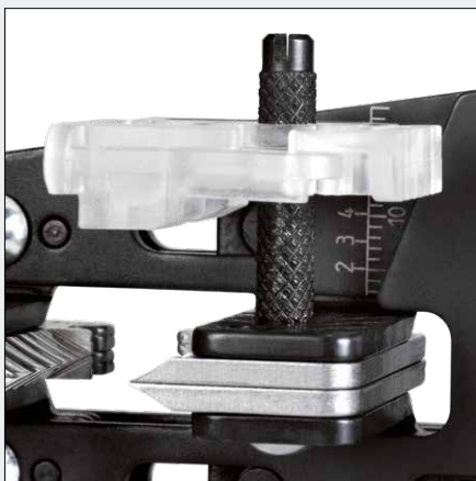
Adjustable length stop with scale
