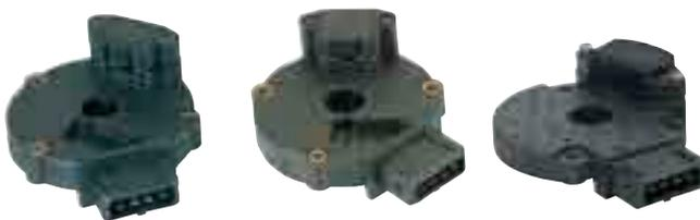
**Optical Sensors** use light switching to generate an output voltage signal indicating crankshaft/camshaft speed and position. The sensor consists of a light source positioned opposite a phototransistor, along with a slotted disc driven by the crankshaft/camshaft.
